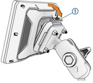
Push the top of the device forward until it snaps into place.The latch 1 on the mount stays up after you have inserted the device.
