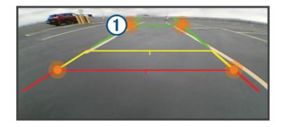
4 If necessary, reposition the vehicle with the other side closely aligned to a kerb, driveway or parking stall lines, and repeat the alignment process.
